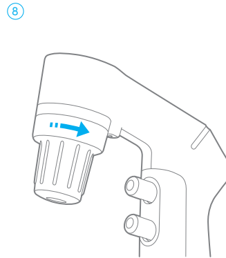
8 Twist the aspiration cone clockwise (do not overtighten).
